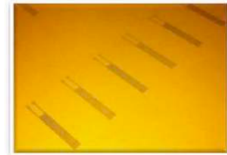
Strain sensor array printed with silver ink
