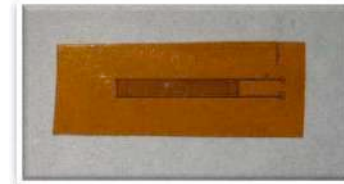
Temperature sensor printed with carbon nanotubes
